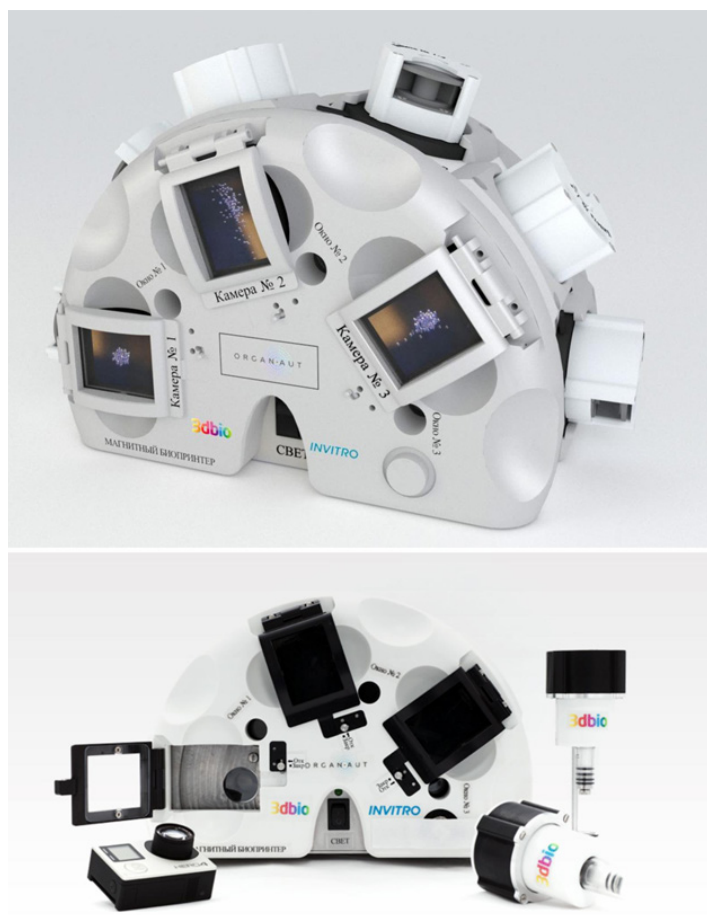
Figure 1. The design (top) and external view (bottom) of magnetic levitational bioassembler Organ.aut from 3D Bioprinting Solutions, Russia. In these designs, “Камера” refers to “camera” and “Окно” refers to “window”. This figure was modified from Parfenov et al. [13], http://creativecommons.org/licenses/by/4.0/
